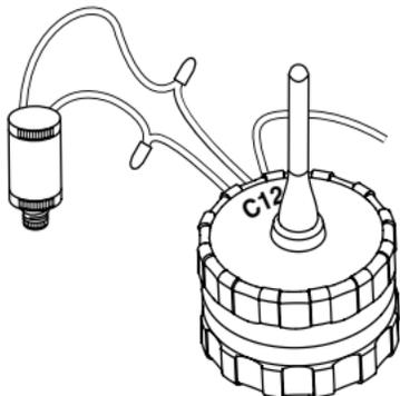
4. Make sure that waterproof connectors are used to secure all wire connections.
