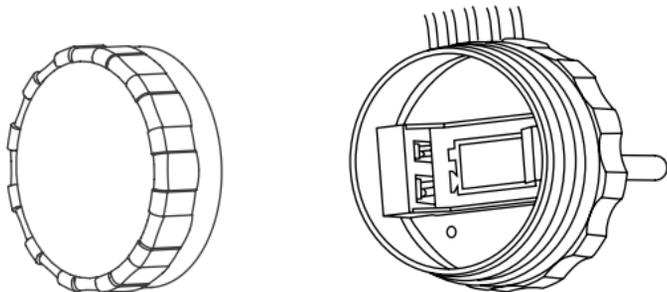
2. Snap the battery into the battery holder.
