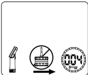
If you are experiencing problems contacting the WVC, make sure you are using the correct identification code. If communication problems persist, try moving closer to the WVC to improve radio contact. The range of the signal will be up to 100 ft. with the WVC installed in the valve box. Actual performance varies depending upon the installation and the
