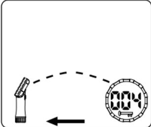
2. Squeeze and hold the Transmit/Receive button on the handle of the WVP for 2 seconds. The WVP will beep twice indicating that communication is taking place.
