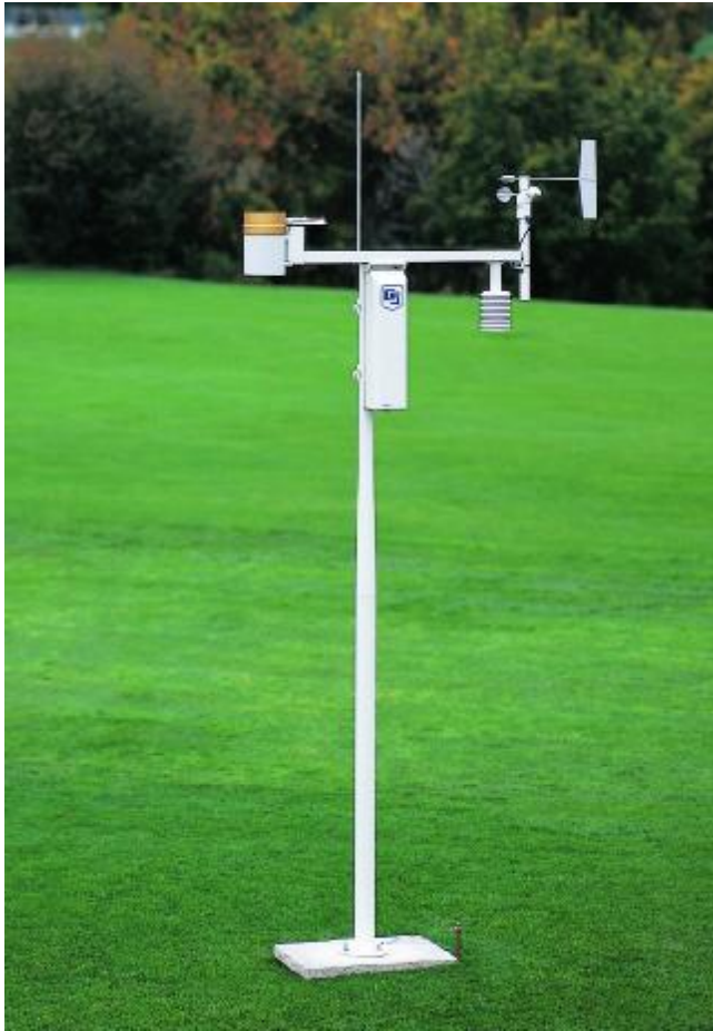
The ET-100 provides real-time weather measurements and calculates ET_0 on an hourly and daily basis.
